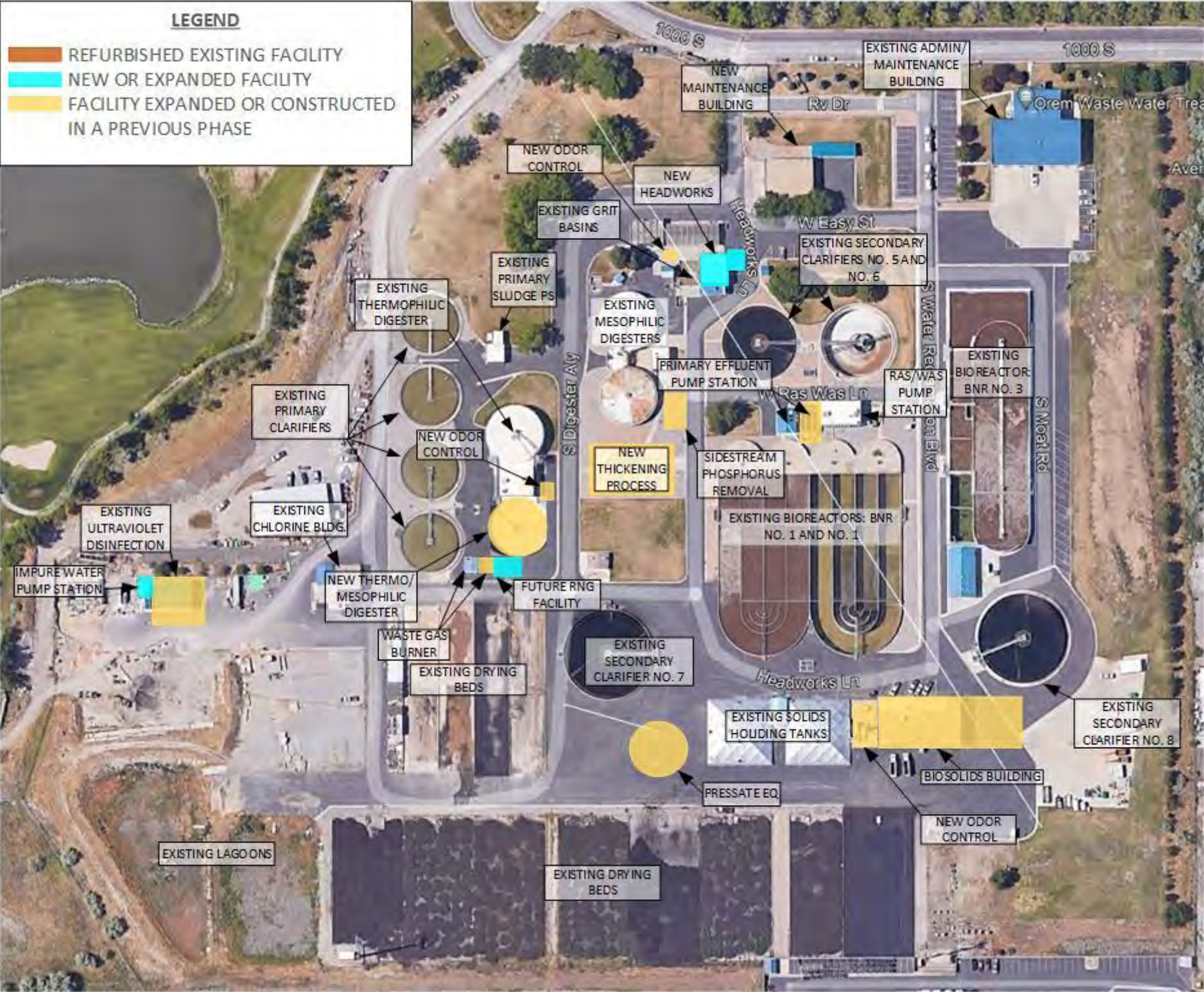
Figure 6-3 – Phase 3 Future OWRF Upgrades
