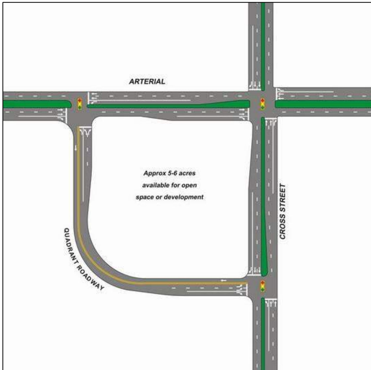
Figure 25: Quadrant Roadway Example
