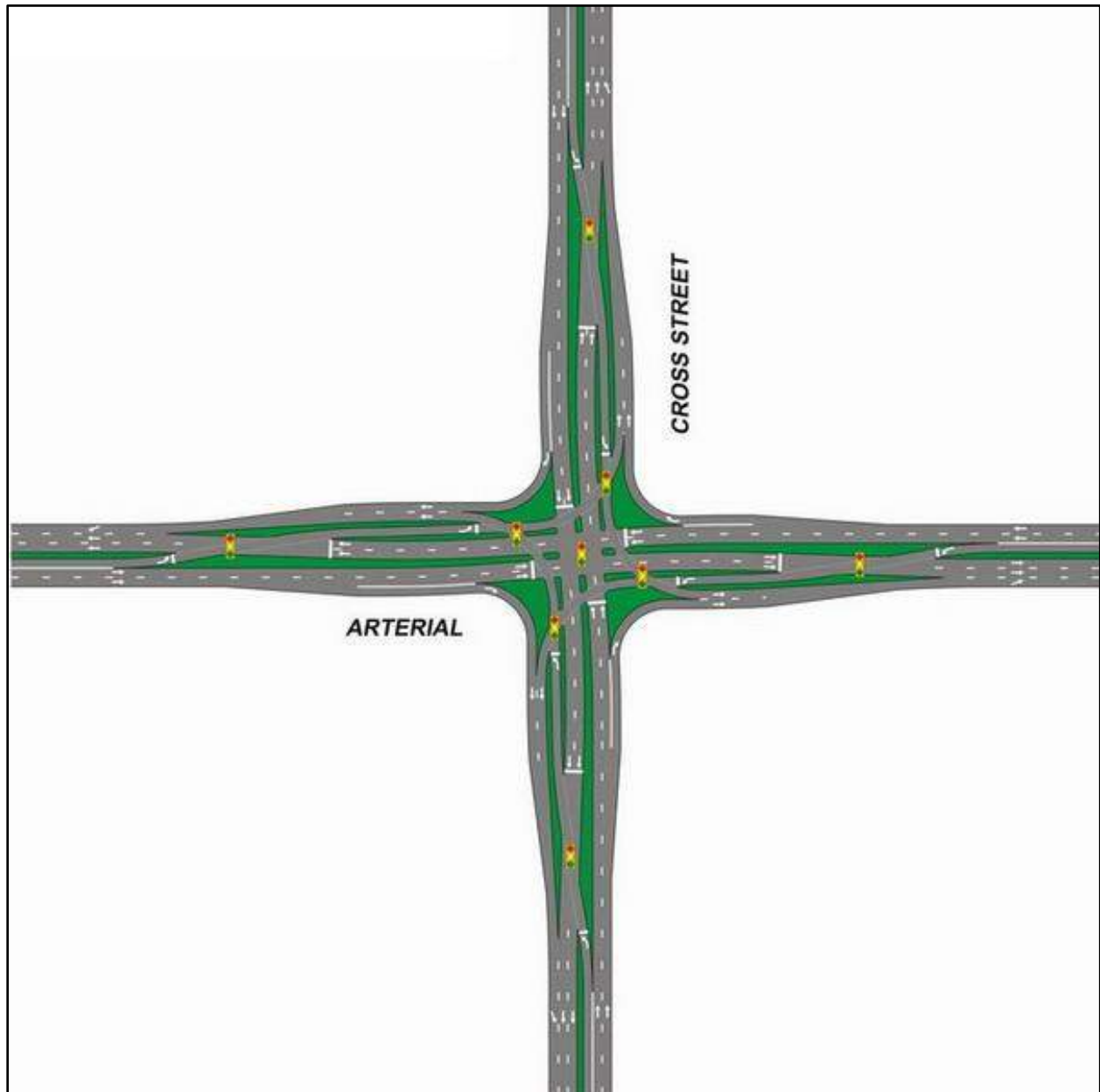
Figure 23: Continuous Flow Intersection (CFI) Example
