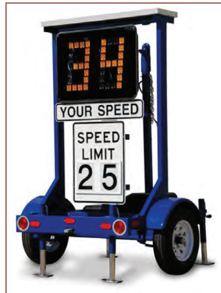
Figure 1: Radar Trailer Device
